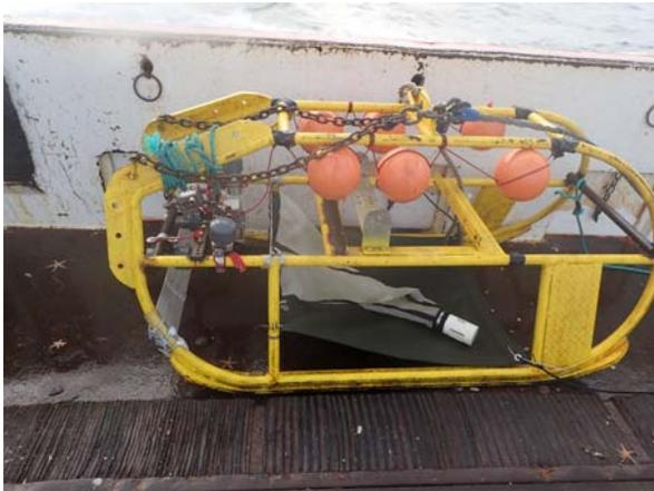
*Figure 6. CFF benthic sled with a plankton net attached inside the frame.*
