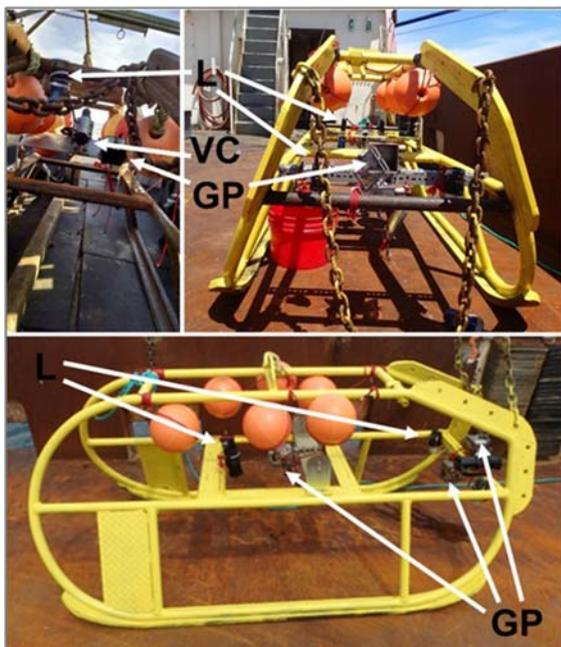
**Figure 5.** On-deck photos of the benthic sled with different camera (VC – Outland Technology underwater camera, GP – waterproof GoPro housings) and light (L – different underwater LED lights) configurations.
