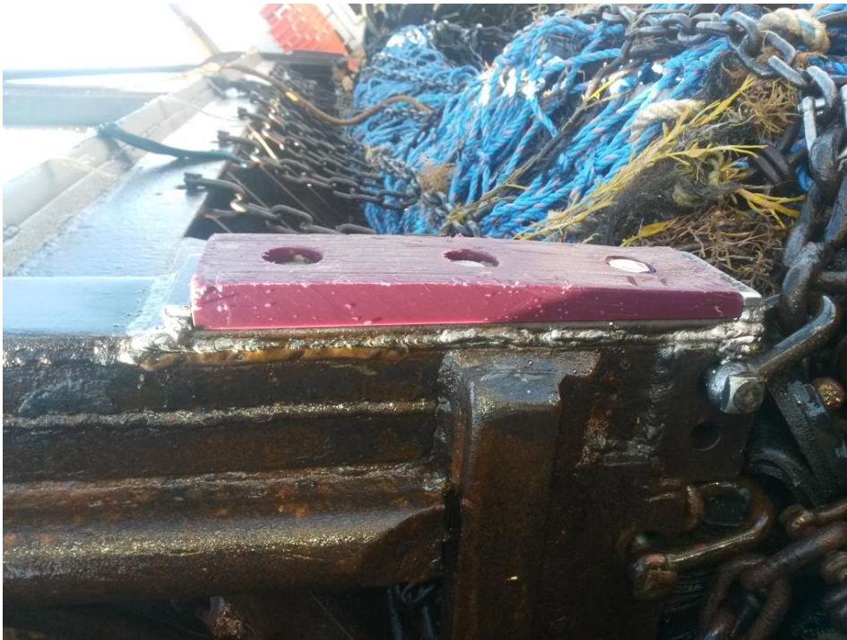
Figure 13: The wear after one 55 minute was too excessive to warrant any further testing of the UHMW plastic shoe.
