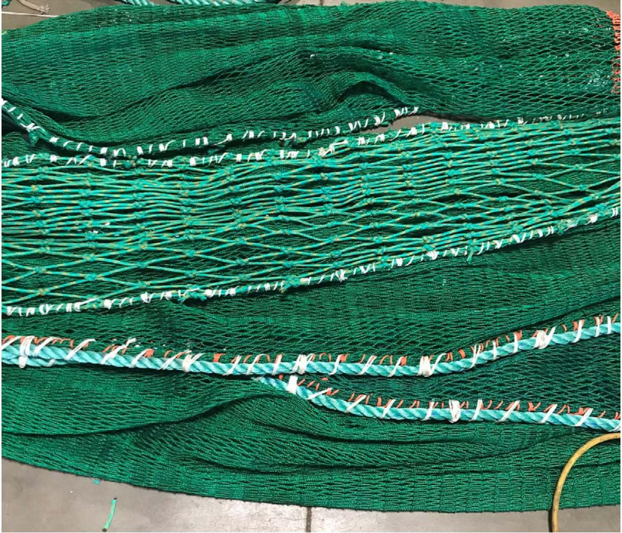
The blowout panel and gore seam reinforcing of the final cover net.
