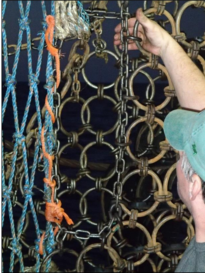
Figure 2 A picture of the CFFTDD14, the dog chain windows, this was the final configuration that was tested during the F/V Celtic , F/V Endeavor and F/V Concordia trips.
