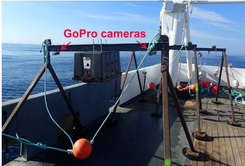
*Figure 1. Camera rig set-up showing three drop camera frames and the locations of the cameras.*
