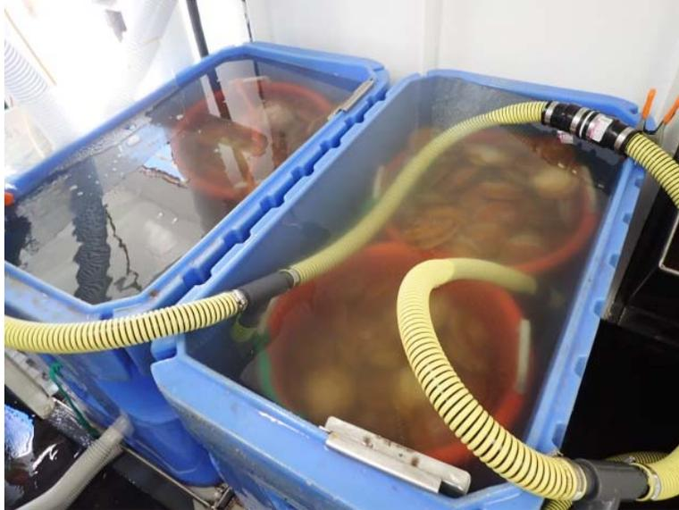
*Figure 3. The cooling system showing two bushel baskets that fit side-by-side in each fish tote.*
