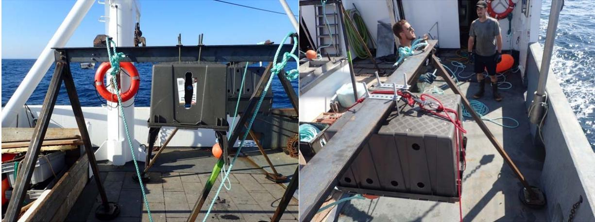
*Figure 5. Close-up views of the quick-release box used to drop scallops onto seafloor in camera view.*
