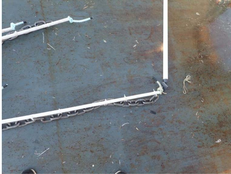
*Figure 6. Tilt current meter attached to a line through PVC pipe.*
